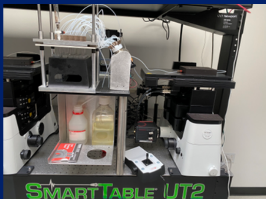
Original fully functional prototype including high resolution microscope and fluidics system attached to a flow cell holding the sample under test.
